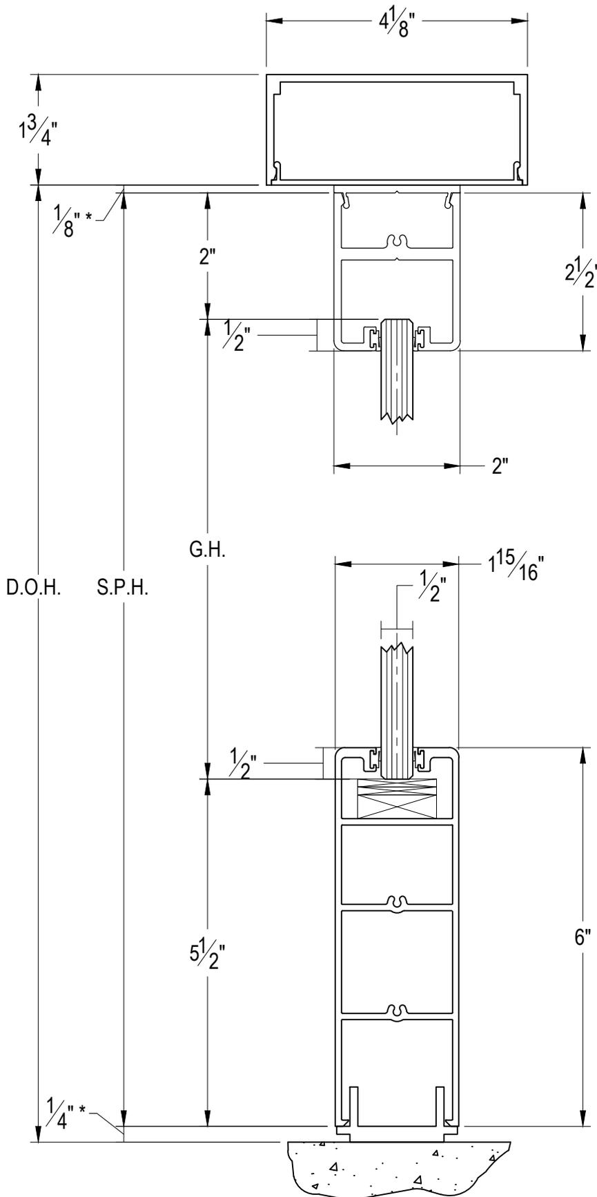
\* OPENING CLEARANCES MAY VARY BASED ON SITE CONDITIONS. STANDARD CLEARANCES SHOWN ARE USED IN FORMULA.
